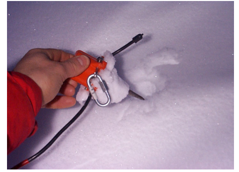
C) Mark's L-15 dual coil geophone.
