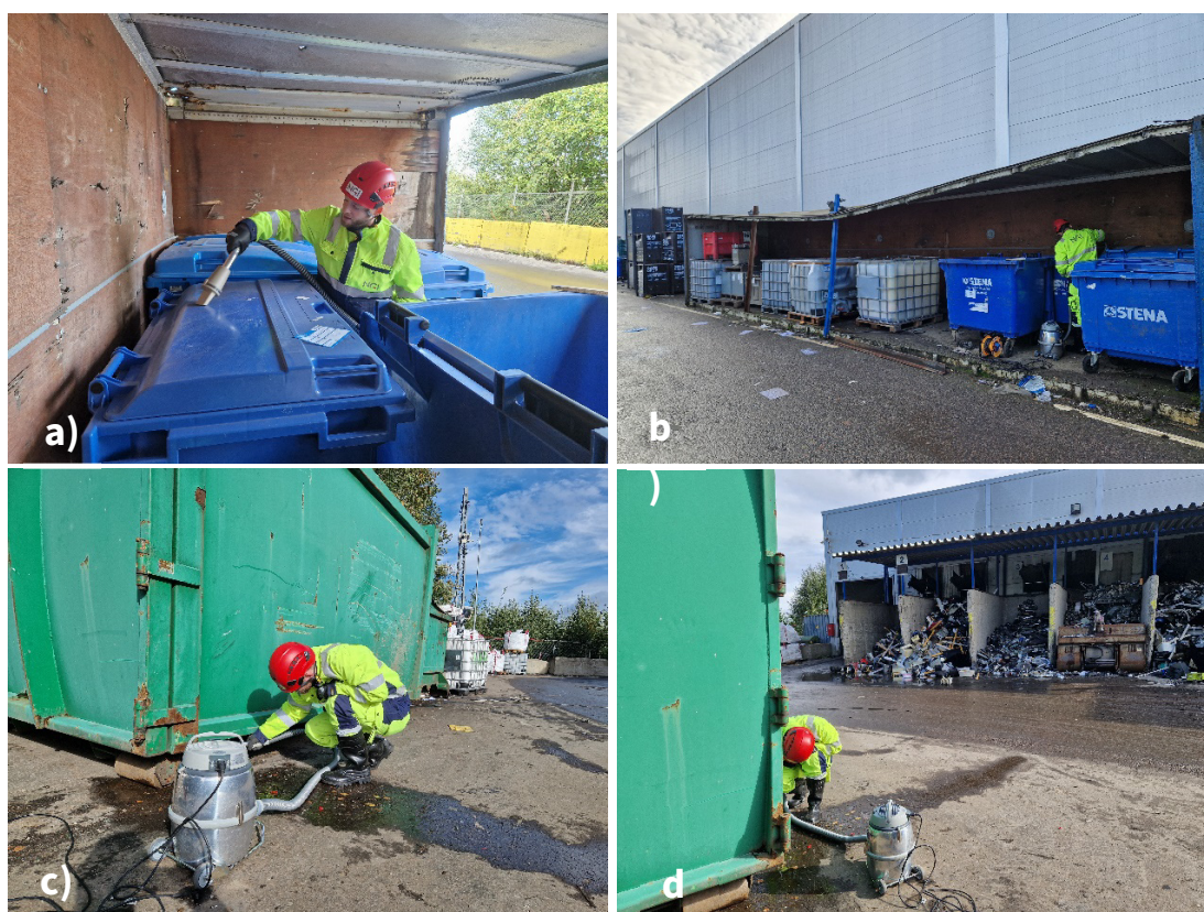
Figure 5: Outdoor dust sampling, EE facility 1.
